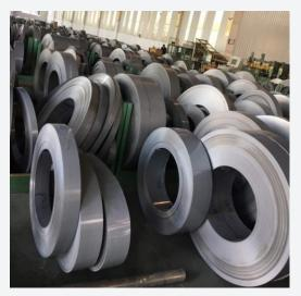
Jaas Steel offers the complete range of CRGO/CRNGO Slit Coils in sizes ranging from 10 mm upwards and thickness ranging from 0.23 mm to 0.30 mm in various grades. These are slit on an slitting machine to attain minimum burr in the cutting edge of the coils, which is typically less than 10 microns.
