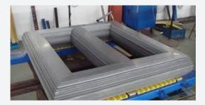
Built Core assembly for transformer with folded/welded frame parts, for 5 KVA to 5MVA. Transformer rating duly tested for No load loss and No load current ready for LV & HV coils insertion.
